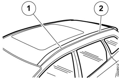
– Position the load carriers on the car roof, approximately at points 1 and 2.
