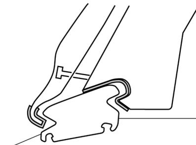
The image shows the correct position of the mounting and the rubber shim around the roof trim strip.
